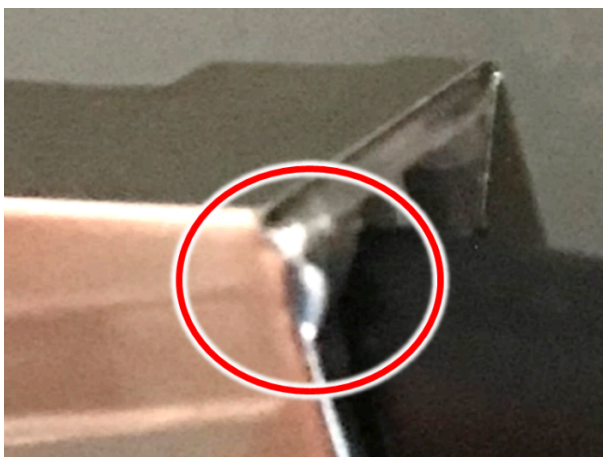
Figure 7. LAN Cable: Shield Wire Soldered to Connector Body
