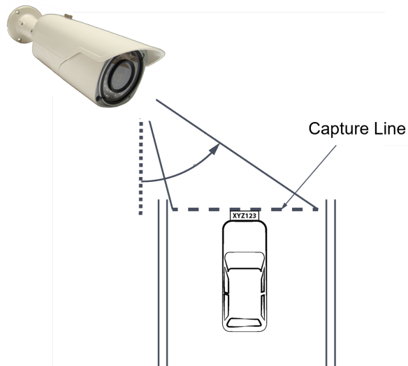
Figure 5. Horizontal Camera Angle (Pan Angle)
