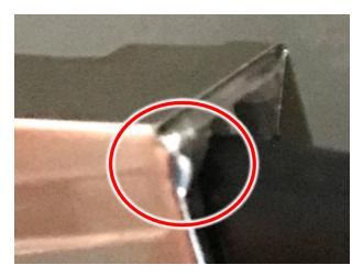
Figure 7. LAN Cable: Shield Wire Soldered to Connector Body
