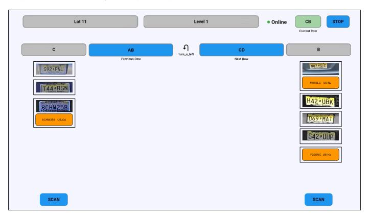
Once the operator finishes scanning, the operator sends the scan result data to IZCloud-PARK. IZCloud-PARK is a modular, cloud-based suite of Automatic License Plate Recognition (ALPR) services. The newly captured scan data is added to the IZCloud-PARK's records, providing a complete current and historical record of parked vehicles, real-time and scheduled pre-generated reports (see the IZCloud-PARK documentation).
