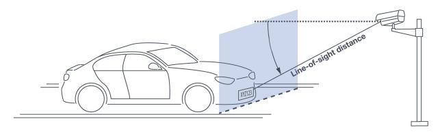
Figure 6. Vertical Camera Angle (Tilt Angle) and Line-of-Sight Distance from Plate
