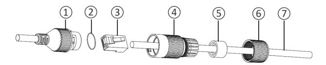
Figure 10. Assembling the Waterproof Cap
