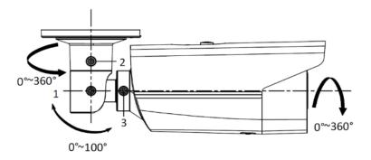
Figure 26. Pan/Tilt/Roll (Angle) Adjustments
