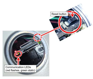
Figure 24. Factory Default (Reset) Button and LEDs
