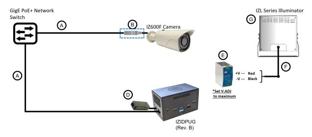
Figure 9. Typical Wiring Diagram
