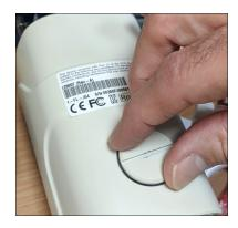
Figure 23. Unscrewing the Round Cover
