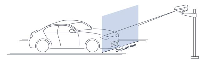
Figure 2. Field of View (Capture Line)
