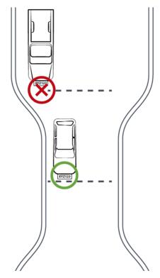
Figure 3. Plates Within Capture Line
