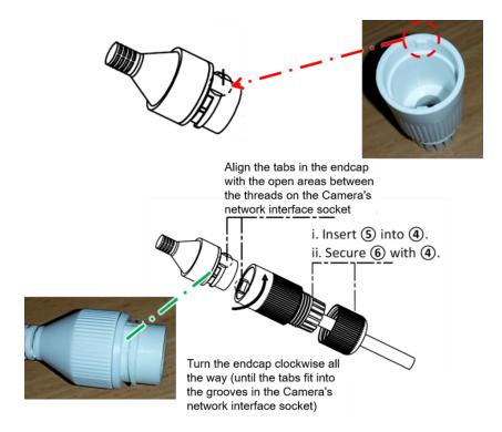
Figure 14. Securing the Waterproof Jacket
