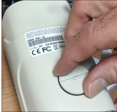
Figure 23. Unscrewing the Round Cover
