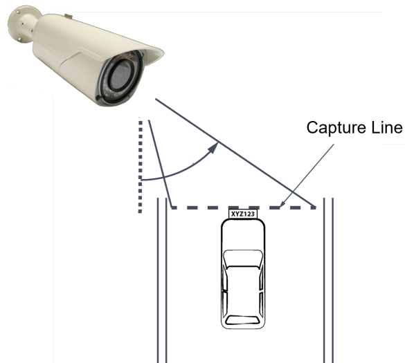
Figure 5. Horizontal Camera Angle (Pan Angle)
