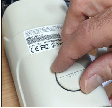
Figure 24. Unscrewing the Round Cover
