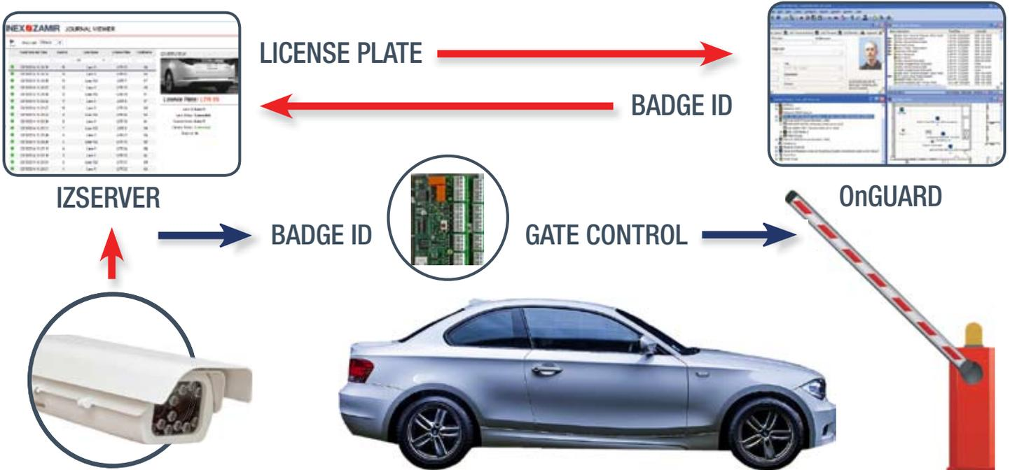
As the vehicle approaches an entry gate, the vehicle's license plate is instantly recognized by the INEX TECHNOLOGIES ALPR Imager, and the system identifies the badge ID of the vehicle operator. The badge ID is then passed to the access control panel over a Wiegand interface in a standard badge
