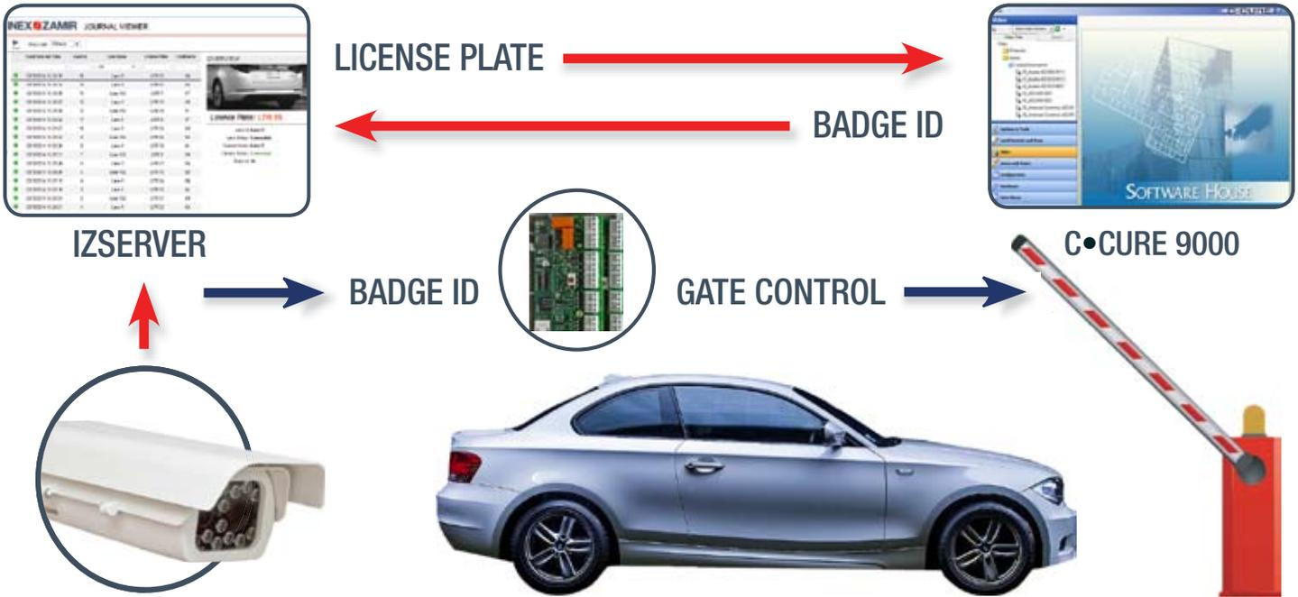
As the vehicle approaches an entry gate, the vehicle's license plate is instantly recognized by the INEX TECHNOLOGIES ALPR Imager, and the system identifies the badge ID of the vehicle operator. The badge ID is then passed to the access control panel over a Wiegand interface in a standard badge
